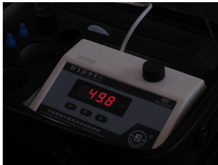
Figure 5: Salt iodine measurement with the WYD spectrophotometer
